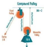
A fixed pulley has a fixed axle, it is used to change the direction of the force on a rope/belt. A fixed pulley has equal force on both sides of the pulley and there is no multiplication of force.
