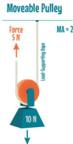
A movable pulley has a free axle - the axle can move in space. Pulling on one end of the rope will apply a doubled force to the object attached to the pulley.
